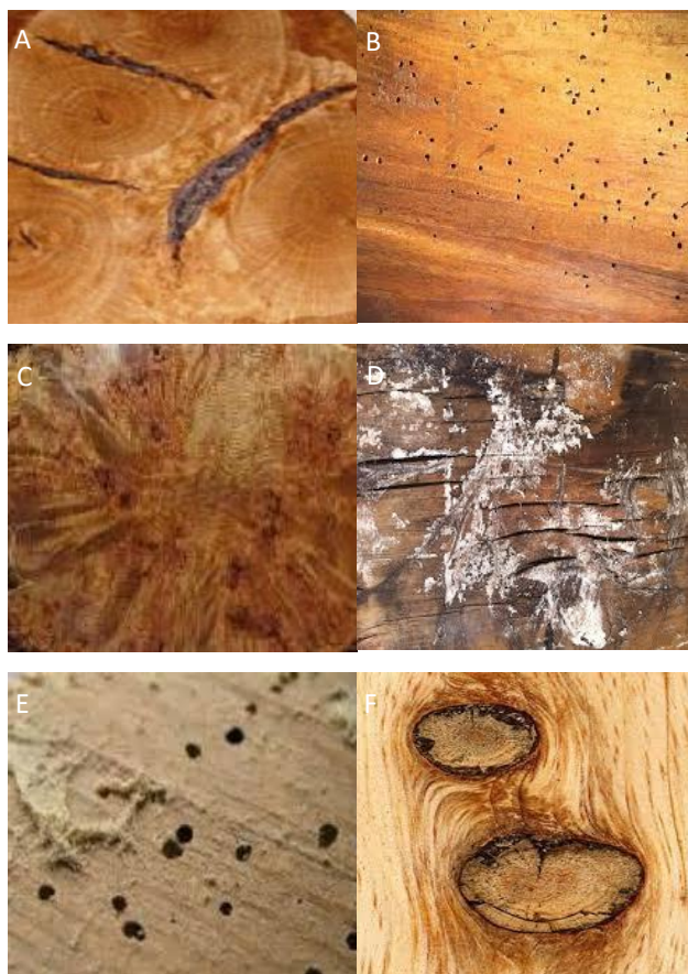
Figure 2. Sample Wood Images a) Bark Pockets b) Bird Pecks c) Burl d) Fungal damage e) Insect defects f) Knot.
