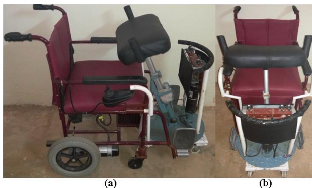
Figure 12. Side view (a) and front view (b) of the powered self-transfer device [20].
