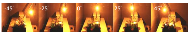
Figure 7. The 2 x 2 pocket sun-tracking system can rotate slowly with the light source.
